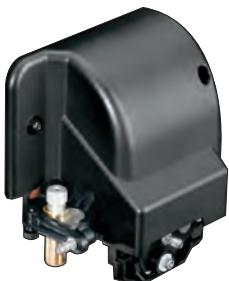
Its simplicity has made **drag knife** (or swivel knife) technology the most commonly used. An offset parameter defines the distance between the knife tip and the rotating centre. In order to know the position of the freely rotating knife inside the knife holder a drag movement is made assuming the knife tip will follow accordingly. Summa cutters include enhanced methods to optimize this drag-movement to obtain the best possible cutting quality.
